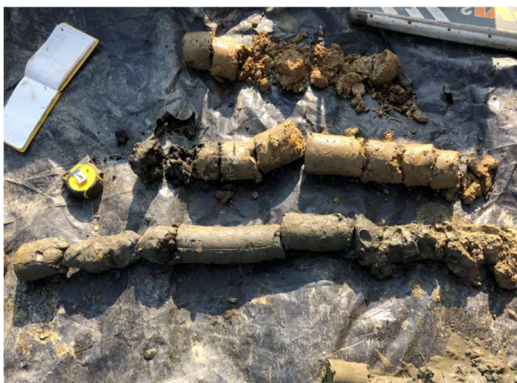
Figure 1: soil arisings from a Window Sampling borehole
