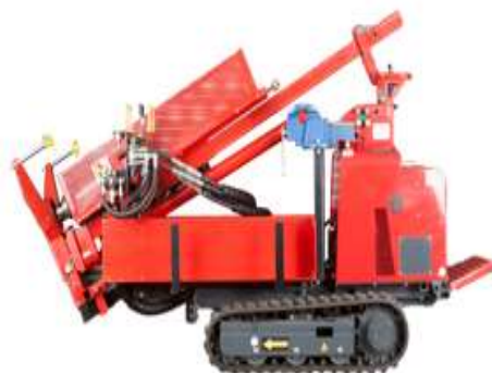
Figure 2: an Archway Dart rig in transport mode
